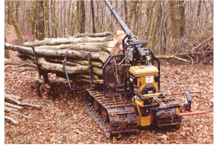
Plate 3. The Oxen, pedestrian controlled forwarder
