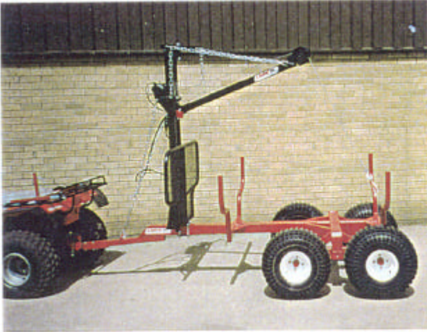
Plate 7 Logic ATV-Equip Timber Trailer with electrically powered wire rope loader
