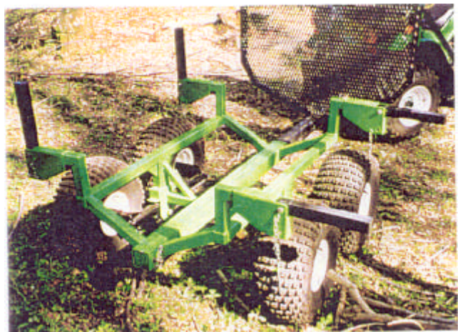
Plate 6. TFM Engineering Multi Role Forestry Trailer with Trailer Body removed enabling forwarder chassis to be used
